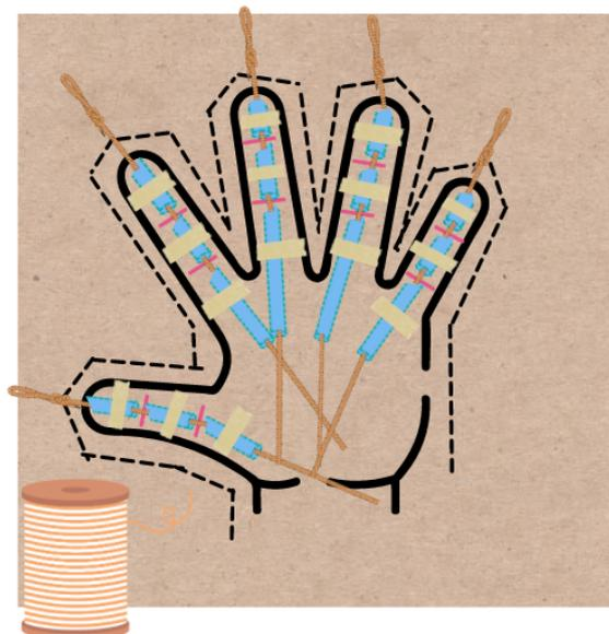
*Figure 5: Five pieces of strings are threaded through the straw pieces on each finger of the hand model.*
